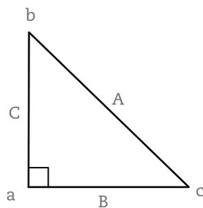
$$\overline{bc}^2 = \overline{ac}^2 + \overline{ab}^2$$
